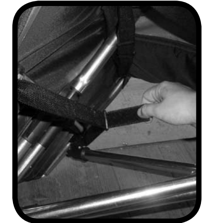
3 Wrap bottom straps around frame, thread strap through D-ring and secure.
