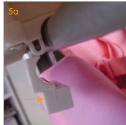
5. Lock the tray as shown (you will hear an audible click)
