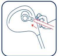
13. Insert the left “A” seat hanger into the motor joint pivot while depressing the button.
