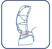
12. Lift the seat assembly and connect the right “B” seat hanger to the swing joint pivot. You will need to depress the button so that the seat hanger will insert into the swing joint pivot completely.
